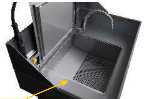
Tank for the soaking of the parts
